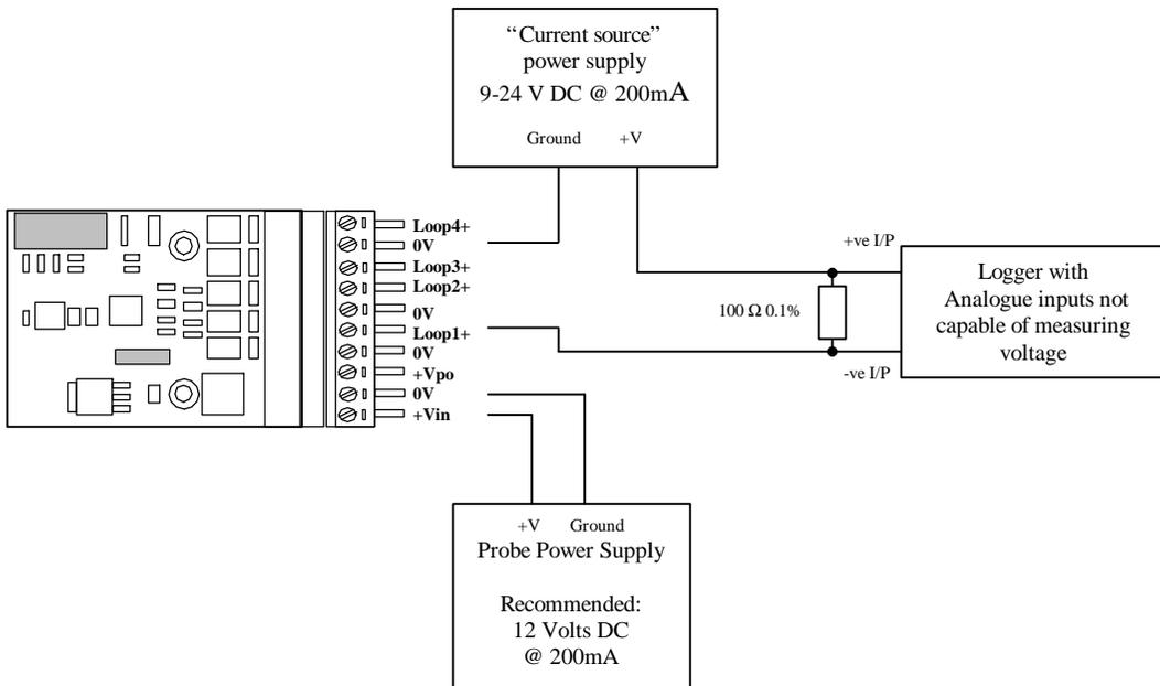
Figure 3: Connection to a logger that only has Voltage measuring capabilities.
