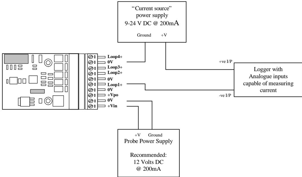
Figure 2: Connection to a logger that has current measuring capabilities.
