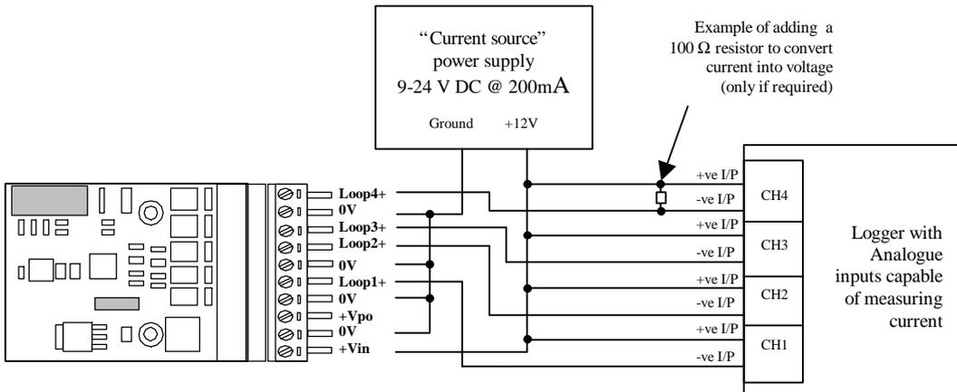
Figure 4: Connection to a logger that has current measuring capabilities using a single supply.
