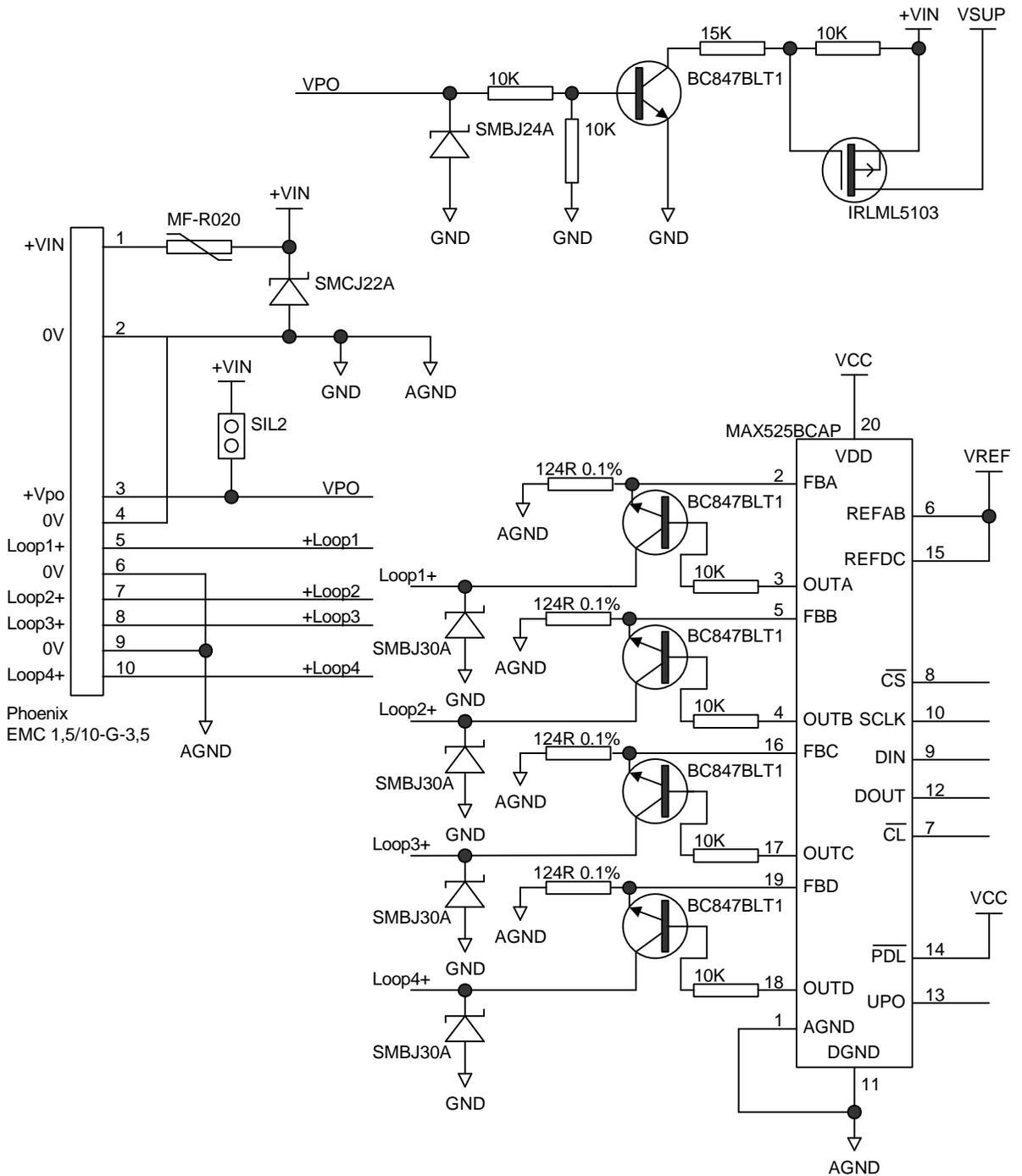
Figure 6: Current interface circuit diagram
