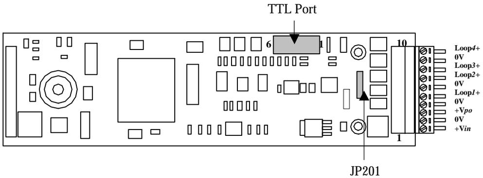
Figure 5: **EnviroSMART** Current probe interface board layout
