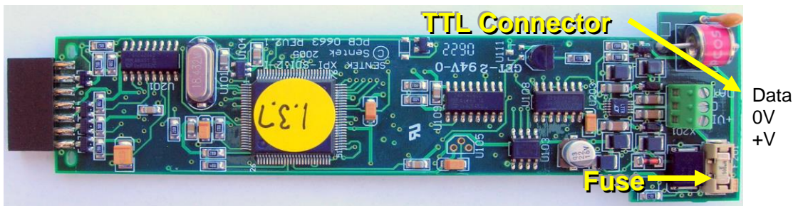
Figure 5 EasyAG SDI-12 probe interface board layout
