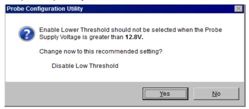
Probe Supply Voltage During operation, this is the voltage as measured by the probe. This measurement is compared to the threshold voltages.
