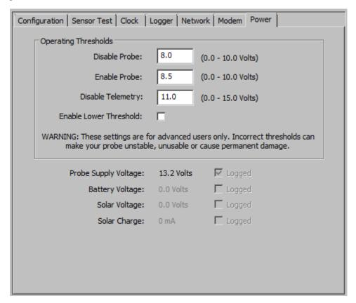
EnviroSCAN Series II and EasyAG Series II probes can operate over a range of voltages from 4 volts to 15 volts. This means they can be powered from different types of power source e.g. batteries. Sentek has done analysis on some typical power sources and has developed suggested values for these thresholds.
