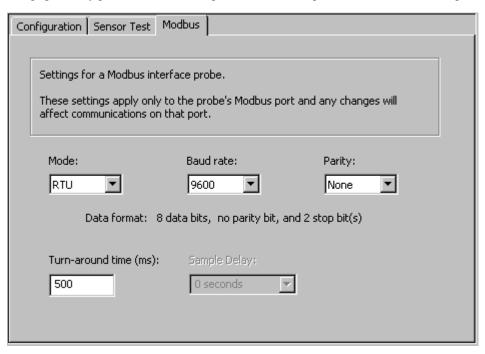
The Modbus page appears if PConfig is connected to a Modbus probe. It enables the setting of the probe's dedicated Modbus communications port's communications parameters.
