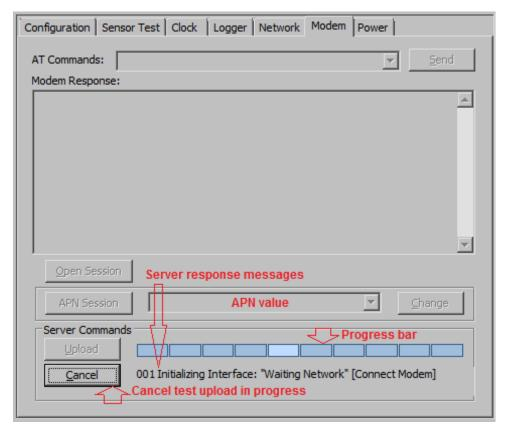
This page requires that the modem be connected to the probe and that the probe and modem have the same baud rate and parity settings. It can be used to setup the modem configuration parameters that cannot be set on the *Logger Page*.
