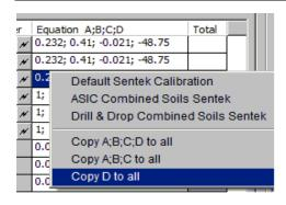
On *Configuration Page* the column "Equation. A;B;C;D" displays the coefficients for each sensor. The fourth value (D) is the temperature compensation value for the moisture sensor.
