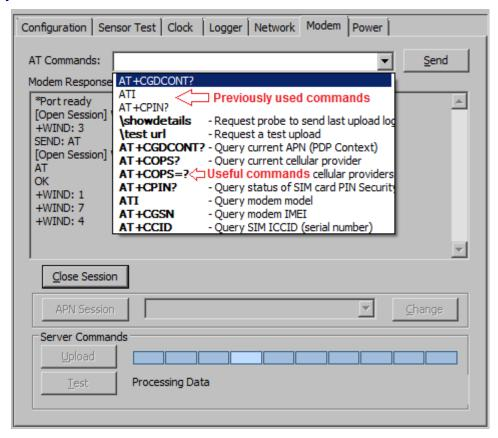
Open Session provides a mechanism for user to send commands to modem, and view what the instant responses will be. The interaction includes **AT Commands** drop-down list, **Send** button, **Modem Response** textbox and **Open Session** button. Click **AT Commands**, to pop up a list of commands which is in two parts. The lower part includes preset useful commands, in bold, defined in the *Configuration File PConfig.ini*. The upper part includes history of the previous sent commands.
