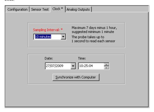
The Clock page is for displaying and changing the probe's sampling interval and clock time. If either of these features is not supported by the probe then the controls related to that feature will be disabled when connected. The color red is used to indicate items that have been modified, and an asterisk appears on the title tab to indicate some change has occurred which has not been written to the probe (this will remain until 'Write To Probe' is used).
