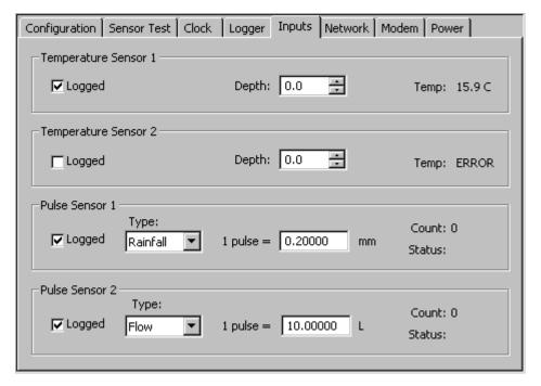
Sentek MULTI supports two temperature sensors and two pulse sensors. It can also optionally log various power values (see *Power Page*)
