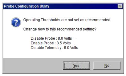
Enable Lower Threshold The Enable Lower Threshold option is used to indicate an acceptable lower Disable Telemetry Operating Threshold and must be set appropriately for the battery type connected to the system. See Disable Telemetry for description of battery types. Only valid with Sentek-PLUS and Sentek-All-in-One.
