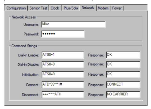
These command strings are used to control a modem connected to the Plus probe.
