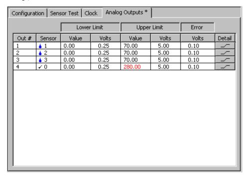
The Analog Outputs page is automatically displayed when a probe with analog outputs is connected (type XPI-5V, XPI-20C etc.). These analog outputs typically produce an output of 0 to 5Vdc or 1-20mAdc (depending on the type of probe), which represent the calibrated value of a sensor.
